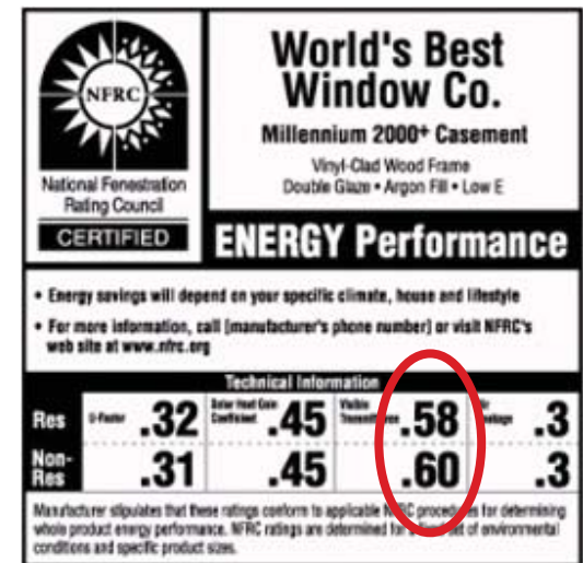
Figure C: Tvis expressed as VT on a window manufacturer's label.
